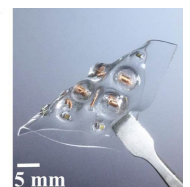
E-skins that can "pulse" in response to pressure. Credit: Wu et al., Sci. Robot. 3, eaat0429 (2018)
