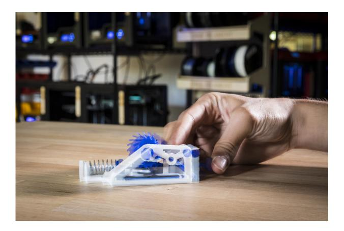
Engineers at the University of Washington created a 3D printed prototype of a device that can store information, such as how many times someone used an insulin pen, by rolling up a spring inside a ratchet that can only move in one direction (shown here). When the user releases the ratchet, the spring unwinds and moves a gear that triggers a switch to contact an antenna. Each contact is counted to determine how many times a person used the device. Credit: Mark Stone/University of Washington
