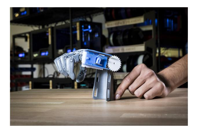
The University of Washington team 3D printed an e-NABLE arm with a prototype of their bidirectional sensor (blue and white) that monitors the hand opening and closing by determining the angle of the wrist. Credit: Mark Stone/University of Washington
