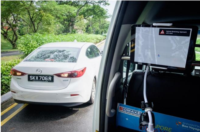
NTU and NXP demonstrated new applications of safety warning systems using V2X, such as alerting the car behind as the car in front reverses. Credit: NTU Singapore
