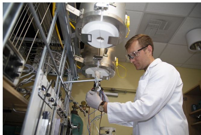
Graduate research assistant Ben deGlee hooks up electrodes to a testing unit used to test the new fuel cell in Meilin Liu's lab at Georgia Tech. Credit: Georgia Tech / Christopher Moore
