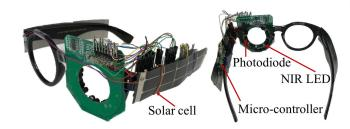
Integrating eye tracker into a regular pair of glasses, the system relies on NIR lights and photodiodes for eye tracking and is powered by two thin solar cells on the arms of the glasses. Credit: DartNets Lab
