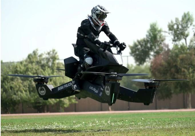
The recommended flight altitude is 5 meters above the ground (16 feet), and [maximum](#) speed is limited to 96 km / h (60 m / Ph).
