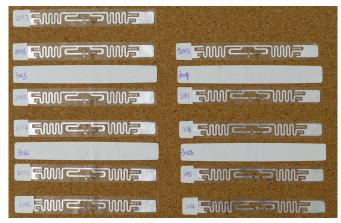
An RFID tag is modified by cutting out a small part its antenna (silver ribbon) and placing a small light-sensing phototransistor or temperature-responsive resistor (thermistor) on it. Credit: University of Waterloo
