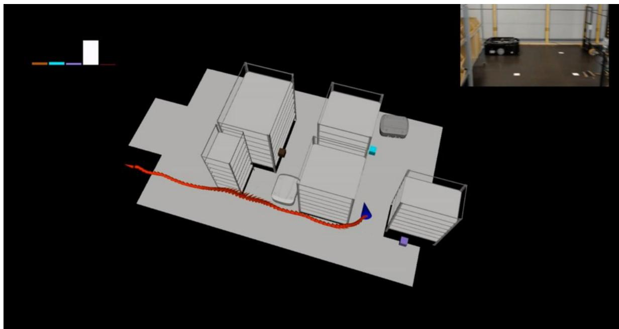
The trajectory of the human worker in the Warehouse test area. The location data is provided by the Hololens' localization algorithm. On the top right the first-person view of the worker can be seen. On the top left are the probabilities of the worker going to a specific goal. Credit: Petkovic et al.
