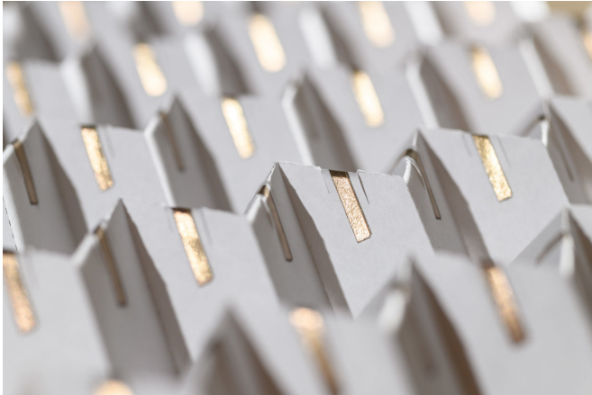
Silver dipoles are arranged across the folds of a Miura-Ori pattern to enable frequency blocking. Credit: Rob Felt
