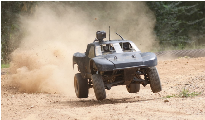
AutoRally vehicle navigating a bump on the track at high speed during testing. Credit: Drews et al.
