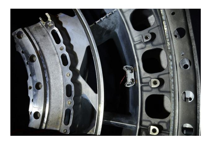
HAMR-E uses electroadhesive pads on its feet and a special gait pattern to climb on vertical, inverted, and on curved surfaces, like the inside of this jet engine. Credit: Wyss Institute at Harvard University
