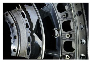
HAMR-E uses electroadhesive pads on its feet and a special gait pattern to climb on vertical, inverted, and on curved surfaces, like the inside of this jet engine. Credit: Wyss Institute at Harvard University
