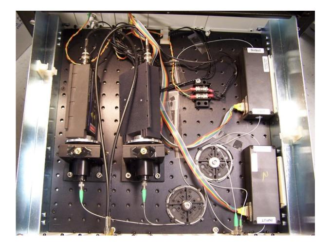
A look inside a prototype of the hardware that exchanges quantum cryptography keys. Credit: <u>National Institute of Standards and Technology/Wikimedia</u>
