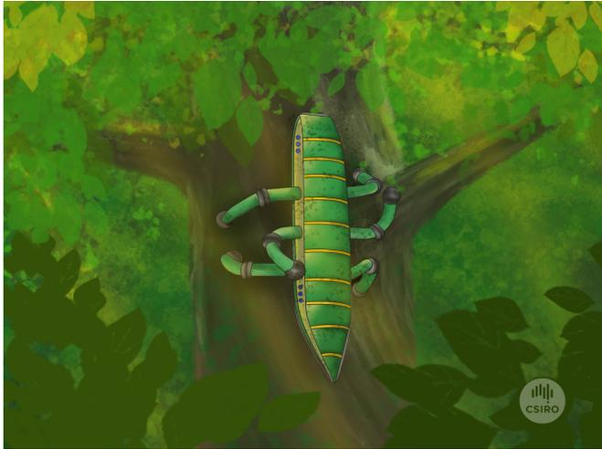
An artist's impression of a robot for use in the Amazon. Based on tree crawling lizards and gecko, it would have articulated legs for more flexibility and climbing. Credit: CSIRO
