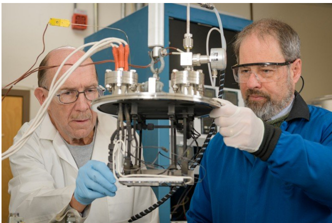
IEC researchers Wayne Buchanan (left) and Brian McCandless (right) lowering the vapor source head into the vapor transport deposition system. Credit: University of Delaware
