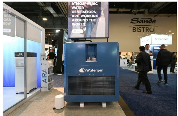
Watergen's GEN-350 machine, which extracts potable water from the air, is seen at the Consumer Electronics Show in Las Vegas
