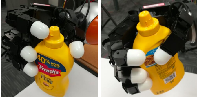
Precision (left) and power (right) grasps generated by the new grasp planner. Credit: Lu & Hermans.
