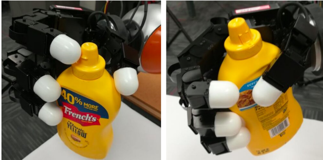
Precision (left) and power (right) grasps generated by the grasp planner. Credit: Lu & Hermans.
