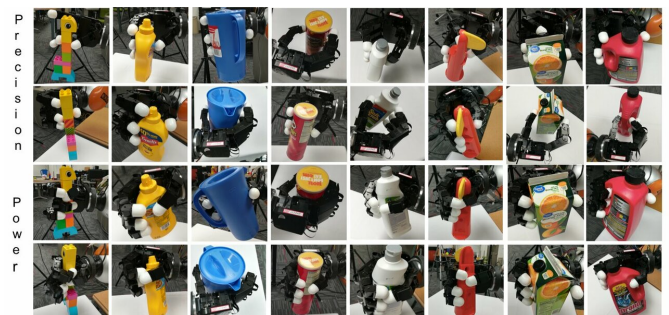
Examples of successful precision and power grasps generated by the new grasp-type modeling approach to grasp planning. The top two rows are precision grasps. The bottom two rows are power grasps. Credit: Lu & Hermans.
