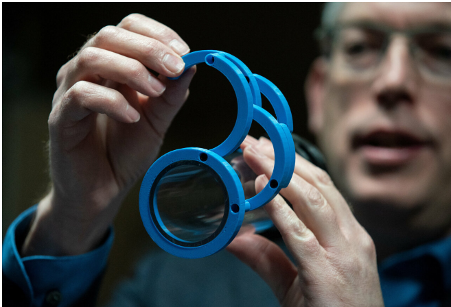
Professor Larry Howell demonstrates the motion on a developable mechanism. Credit: BYU
