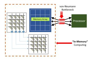
This is an illustration of the von-Neumann bottleneck. Frequent to-and-fro data transfers between the processor and memory units incur large energy consumption and limit the throughput. 'In-memory computing' allows performing computations on the data they store within, thereby reducing the number of unnecessary transfers of data to the processor. Credit: Purdue University
