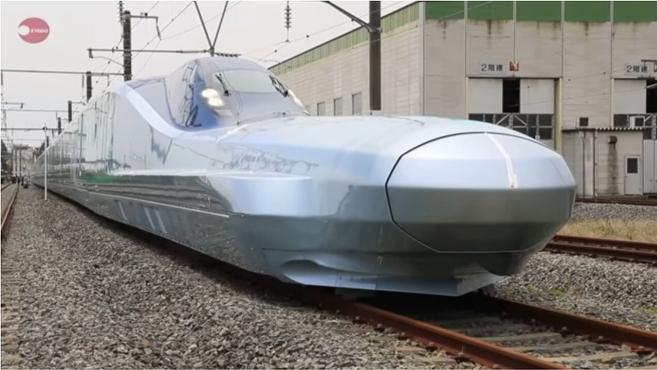
Testing for a train capable of 249mph (400 kph) speeds is to happen about twice a week at night. Bloomberg said ALFA-X is the world's fastest bullet train— well, for now, it is holding that title. Japan has also been working on a maglev train.
