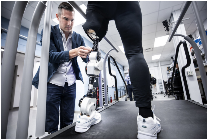
Elliott Rouse, Assistant Professor of Mechanical Engineering, runs tests on an open-source robotic leg with Dawn Jordan Musil. Credit: Joseph Xu, Michigan Engineering
