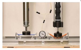
The team showed in an object-crushing comparison between a conventional piston (air cylinder; left) and a tension piston (right) that the tension piston can produce greater forces at the same air-pressure. Credit: Wyss Institute at Harvard University
