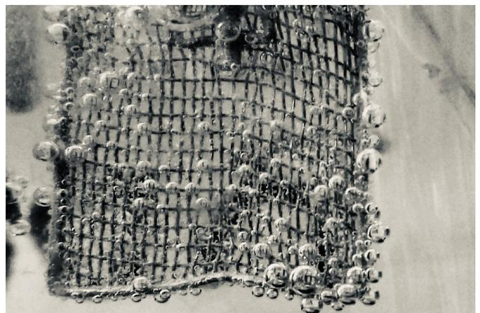
Hydrogen bubbles formed through the water splitting reaction via magnetic enhancement. Credit: ICIQ
