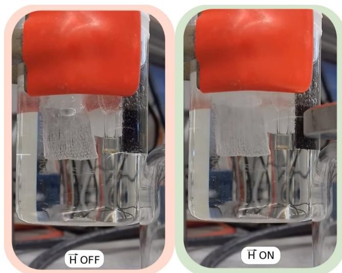
There's an observable increase in the hydrogen bubble formation when the magnet is approached to the anode. Credit: ICIQ
