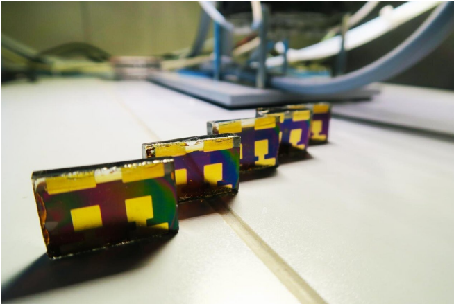
Perovskite solar cells in the lab. Credit: Wolfgang Tress (EPFL)
