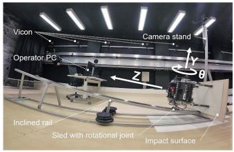
Test rigs for <u>SpaceBok</u> have been set up to simulate various gravity environments, mimicking not only lunar conditions but the very low gravities of asteroids. The lower the gravity the longer the flight phase can be for each robot jump, but effective control is needed for both take-off and landing. Credit: ETH Zurich/ZHAW Zurich
