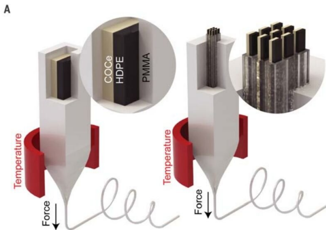
Bimorph fibers produced via two-step thermal drawing. HDPE, high density PE. Credit: Science (2019). 10.1126/science.aaw2502
