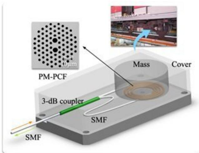
The new fiber-optic accelerometer features a polarization-maintaining photonic crystal fiber that is coiled into the shape of a disc only 15 millimeters in diameter. When a vibration occurs, the mass block presses on the coiled fiber at a frequency matching that of the vibration. This external force causes the wavelength of light in the fiber to shift in a measurable way. Credit: The Hong Kong Polytechnic University
