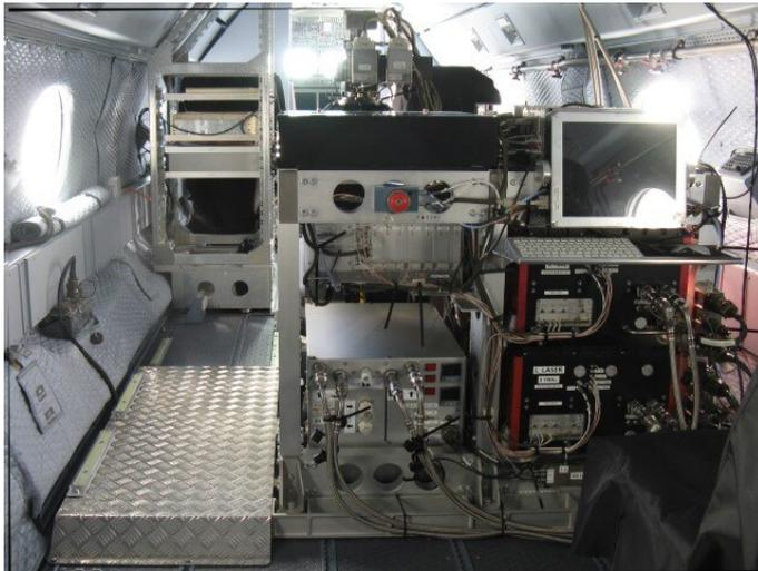
The new lidar system was used for airborne atmospheric measurements during the wave-driven isentropic exchange (WISE) mission, which involved multiple long-range flights over the North Atlantic and Northern Europe. Credit: DLR
