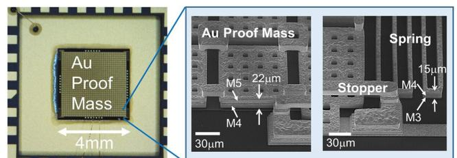
Left; The photo shows a developed high-sensitivity MEMS Accelerometer. The Au proof mass was fabricated on a silicon die. The accelerometer was implemented in a ceramic package and wire-bonded. Right; The SEM images show the close-up views of the Au proof mass and the spring structure. The Au proof-mass structure of 22-µm thickness was successfully developed by employing the M4 and M5 layers. The serpentine spring
