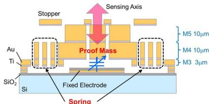
The illustration shows a schematic image of the proposed single-axis MEMS capacitive accelerometer. Input acceleration can be sensed by monitoring the capacitance change between the proof mass and the fixed electrode. The device is realized by the multiple layers made of electroplated gold. We utilize the third (M3) and fourth (M4) layers for the spring structure, and the M4 and fifth (M5) layers for the proof mass structure. Credit: Sensors and Materials, Daisuke Yamane
