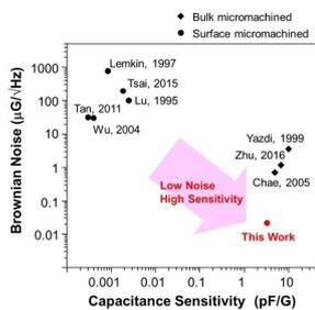
The graph shows a comparison of Brownian noise (BN) versus capacitance sensitivity. Thanks to the high density
