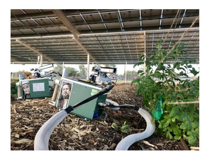
Researchers test the heat and moisture under the solar panels to study the cooling relationship between the crops and panels. Credit: Greg Barron-Gafford
