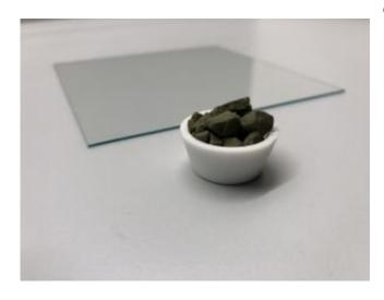
Transparent, electrically conductive, and selective to one type of charge carriers: these are the properties of hole transport layers for Perovskite solar cells. Credit: Tobias Abzieher, KIT
