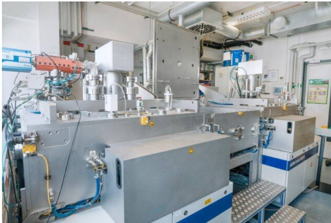
Chemical vapor deposition (CVD) coating plant used to produce functionalized textiles. Credit: © Fraunhofer IKTS
