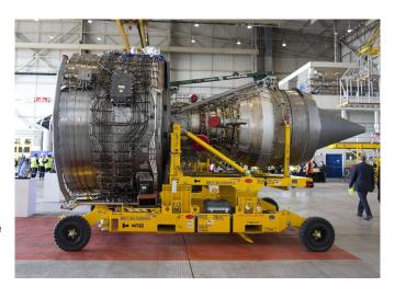
Some parts of the Trent 1000 turbofan engine have worn out more quickly than expected, leading to costly repairs for Rolls Royce
