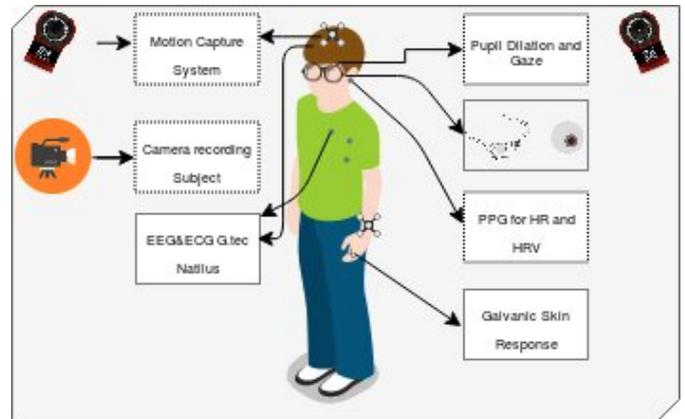
Sensors and devices used in the prototype implementation. The researchers used a motion capture system to monitor human motion and a camera to record the experiment. They also tracked human-gaze using Pupil Labs and human physiological responses such as pupil dilation, PPG, GSR, EEG \& ECG recorded. Credit: Savur, Kumar & Sahin.
