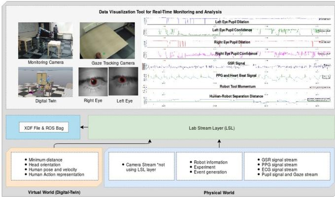
A system diagram of the implementation based on the proposed framework representing the data collection and monitoring during an HRC experiment. Credit: Savur, Kumar & Sahin.
