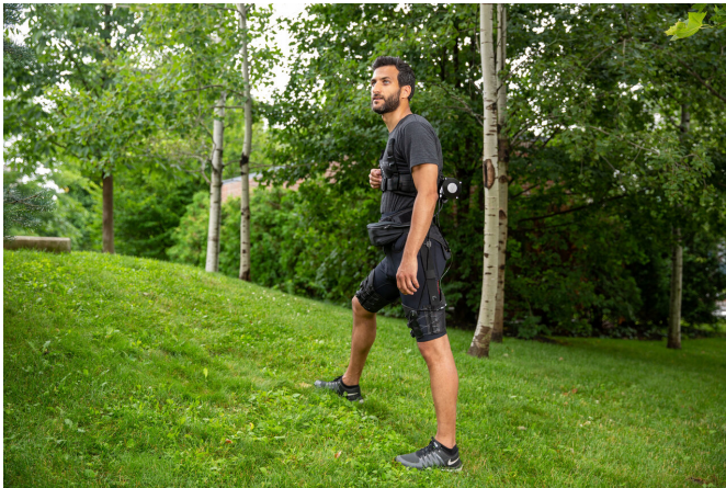
The light-weight versatile exosuit assists hip extension during uphill walking, and at different running speeds in natural terrain. Credit: Wyss Institute at Harvard University
