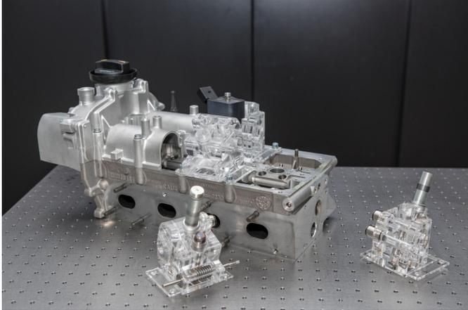
Model of the FlexWork valve drive, mounted on a series production engine. Credit: Empa
