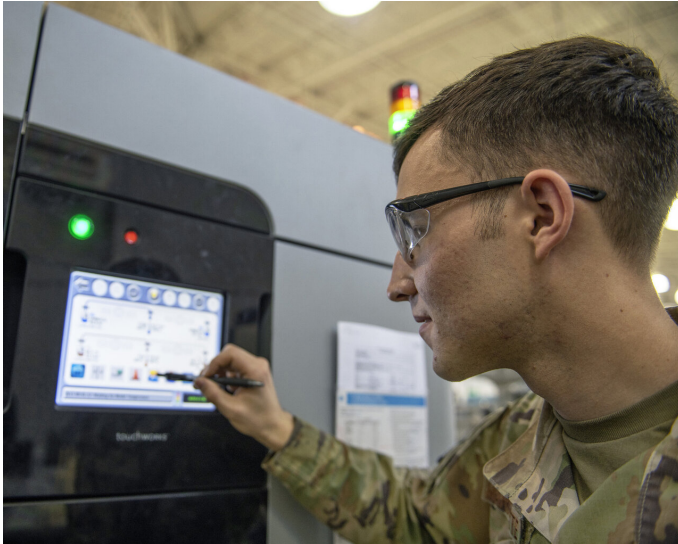
U.S. Air Force Senior Airman Noah Marconette, 60th Maintenance Squadron aircraft metals apprentice loads up a job on the Stratasys F900 three-dimensional printer Aug. 15, 2019 at Travis Air Force Base, California. Travis AFB is the first-unit level location in the Air Force to have the Stratasys F900 3-D industrial printer certified by the Federal Aviation Administration and Air Force Advanced Technology and Training Center for use on aircraft replacement parts. Credit: U.S. Air Force photo by Louis Briscese
