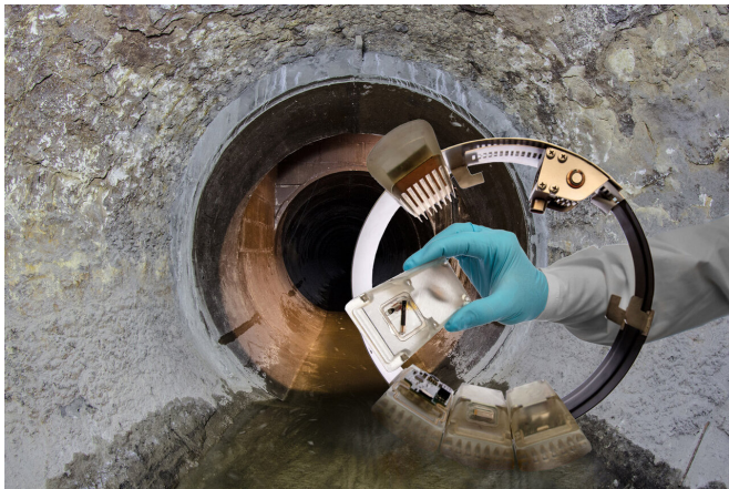
Sensor ring for use in wastewater treatment plants. Credit: Volker Mai
