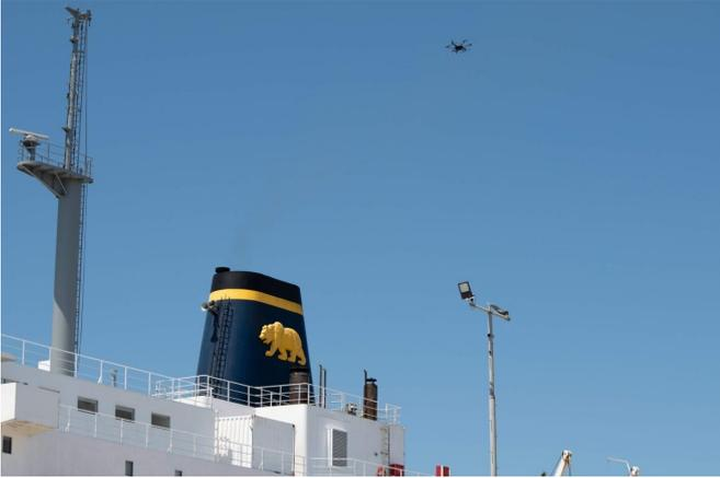
A drone hovers in the exhaust plume of the TS Golden Bear to test a new system for monitoring fuel standards. Credit: Nicki Aviel/UCLA
