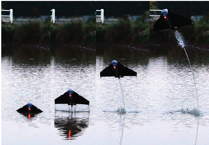
Composite image of the robot in floating, jetting and flying mode. Credit: Zufferey et al., Sci. Robot. 4, eaax7330 (2019)
