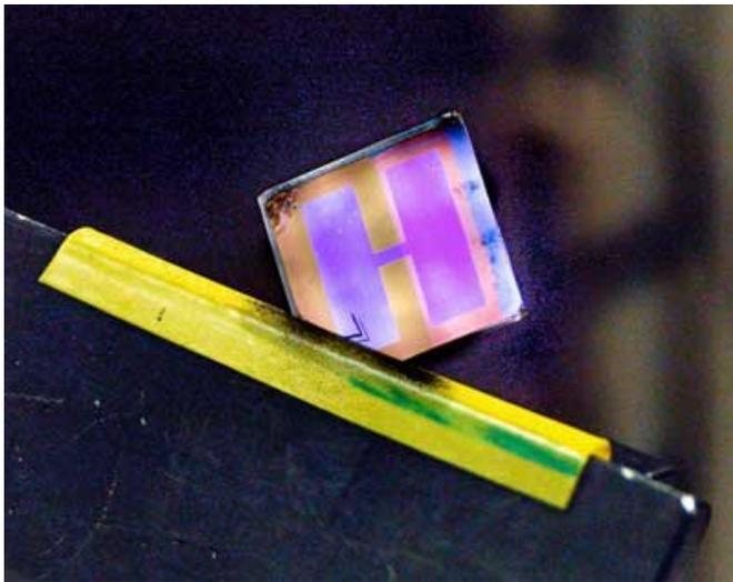
The organic solar cell optimised to convert ambient indoor light to electricity. Credit: Thor Balkhed
