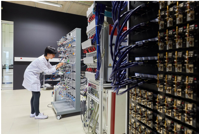
Testing coin cells at battery tester. Credit: CIC energigUNE
