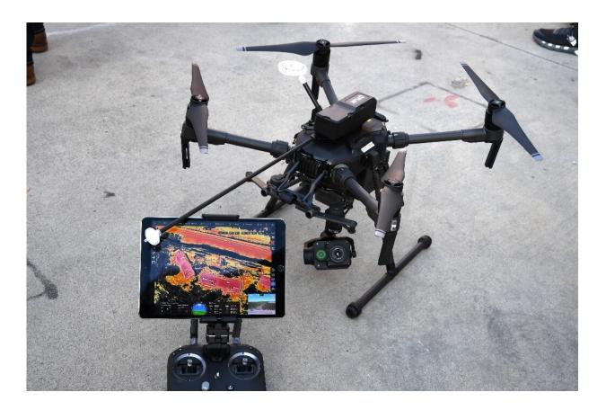
The FLIR C360 Muve gas detector, seen on a DJI Matrice 210 drone, can map toxic gases for the fire and emergency services
