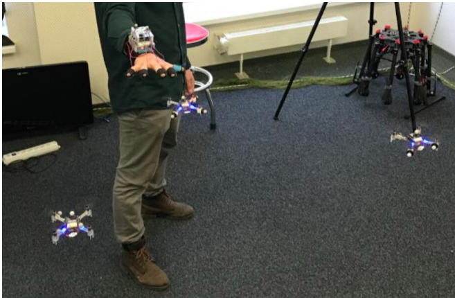
A user manipulating the formation of a swarm of drones using SwarmTouch. Credit: Tsykunov et al.
