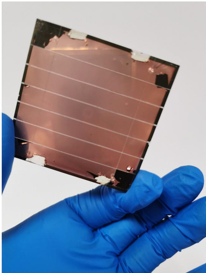
A photograph of an all-perovskite tandem solar cell fabricated by the researchers. Credit: Lin et al.
