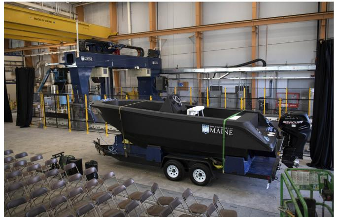
In this Wednesday, Oct. 9, 2019 photo provided by the University of Maine, a 25-foot, 5,000-pound patrol boat, center, that was produced using a large polymer 3D printer, behind left, rests on a trailer on the school's campus, in Orono, Maine. The boat was printed at the school's Composites Center on the world's largest polymer 3D printer. (Ron Lisnet/University of Maine via AP)
