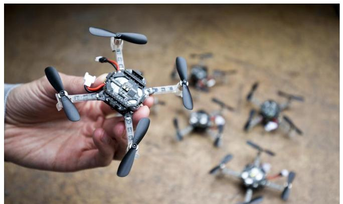
The tiny drone fits into the palm of a hand and weighs 33 grams. Together with the other drones in a swarm, it is able to quickly explore an unmanned environment.
