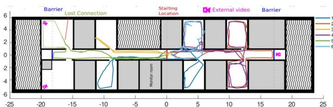
Trajectories of 6 tiny drones exploring an entire office floor in less than 6 minutes. The drones first fly away from the base station at the starting location in the middle, explore the open rooms, and finally return to the base station
