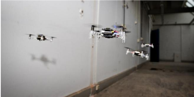
The drones explore the environment by flying into different directions. When a drone notices another drone in its preferred direction, it will attempt to fly in a different direction. When this is not possible (as in this picture), the lower priority drones will move out of the way of the higher priority drones. Drones deal with obstacles on the fly, and by doing so enter and exit different rooms. Credit: TU Delft/ MAVLab
