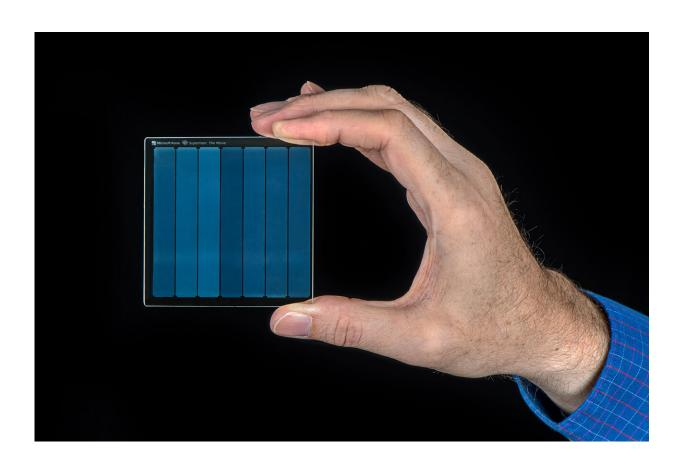
In a proof of concept test for Project Silica, Microsoft and Warner Bros. have successfully stored and read back the classic 1978 "Superman" movie on a 7.5 cm x 7.5 cm x 2 mm piece of durable silica glass — roughly the size of a drink coaster. The glass contains 75.6 GB of data plus error redundancy codes. Credit: Jonathan Banks for Microsoft.
