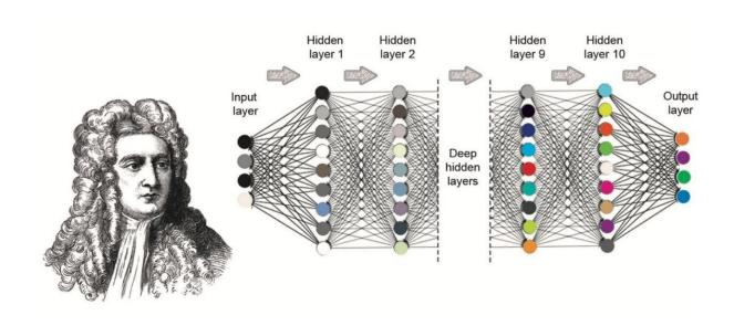
Newton and the machine. Image of sir Isaac Newton alongside a schematic of a 10-layer deep neural network. In each layer (apart from the input layer), a node takes the weighted input from the previous layer's nodes (plus a bias) and then applies an activation function before passing data to the next node. The weights (and bias) are free parameters which are updated during training. Credit: arXiv:1910.07291 [astro-ph.GA]
