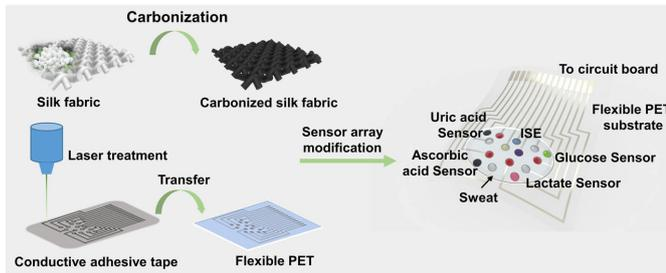
Schematic illustration of fabrication process of the sensor patch. Credit: Tsinghua University
