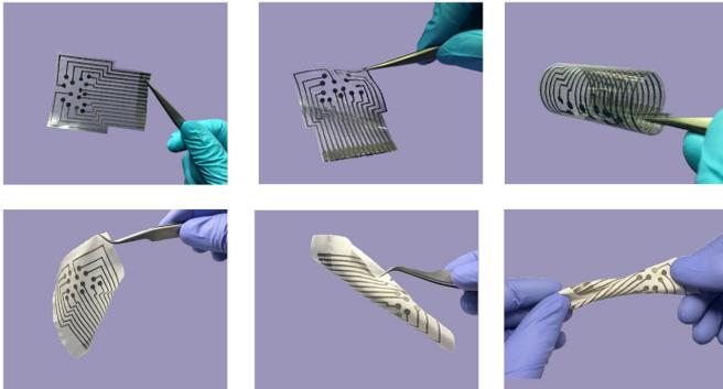
Sensor array on different flexible substrates. Credit: Tsinghua University
