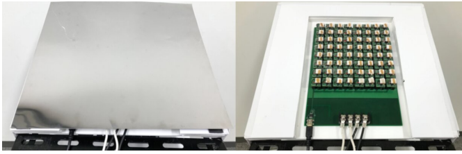
Fig. 3. StickyTouch covered with a stainless-steel plate (left) and StickyTouch uncovered (right). Credit: Osaka University
